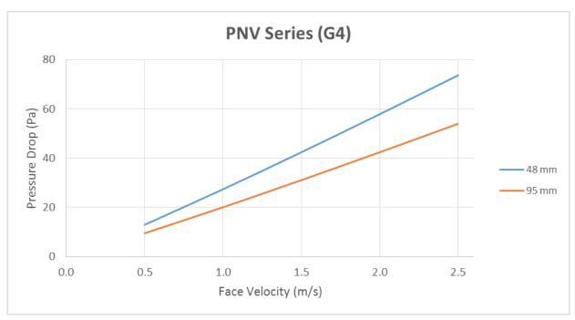
Data based on clean air flow at 25°C. Applies for standard Pleated Panel Filters of G4 media. This graph should be used for guidance only and its accuracy is dependent on the application. The final suitability of the filter is the sole responsibility of the user(s).
